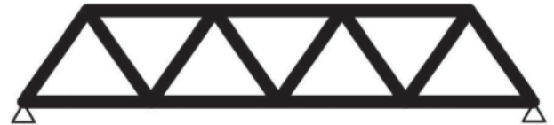
Warren truss architecture is a series of repeated triangular sections. When used in a bridge some of the diagonal elements are in compression and others are in tension.
