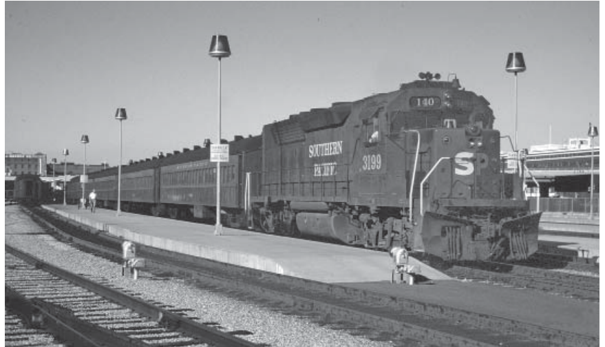
Unique peninsula commute power, GP40P-2 #3199 was one of only three ordered specifically for this service. Here it waits in San Francisco to hustle train #140 timetable East (compass South) in June of 1981. The single-level “suburban” commute cars remained in service long after the first bilevel cars arrived in 1955. Mark Llanuza photo.
